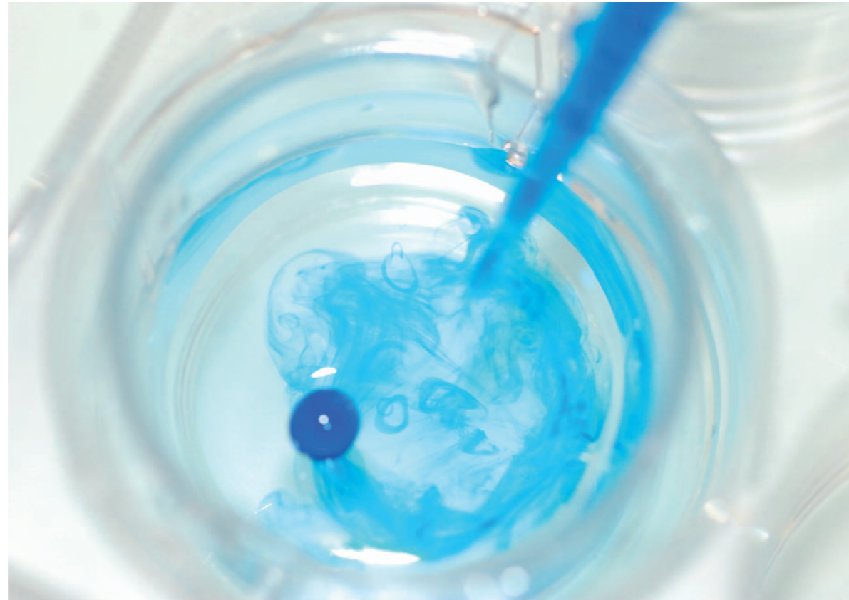
Fig. 3: The passage of blue dextran from the upper to the lower chamber is used to assess epithelial-endothelial bilayer integrity.
