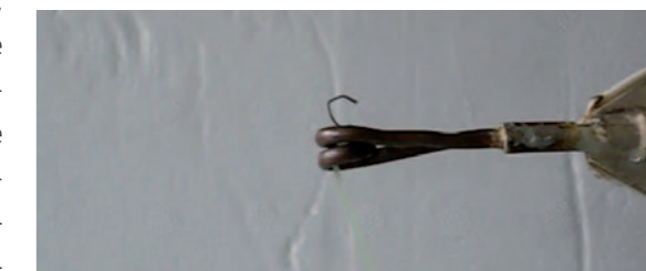
Shape recovery of a polymer nanocomposite strip upon application of an oscillating magnetic field.
