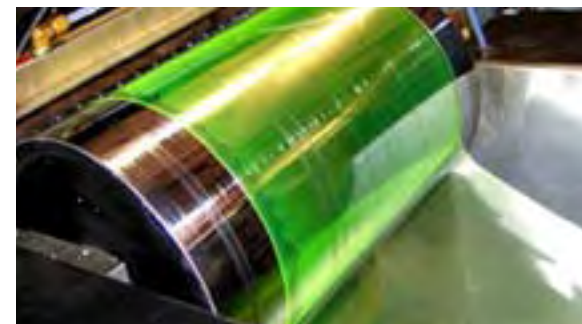
Roll-to-roll manufacturing of a multilayer Laser film.
