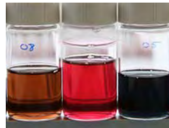
Figure 5: Aqueous dispersions of gold nanoparticles with different shape, colour is dependent on the shape.
