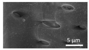
Scanning electron micrograph of nanoparticles in a beech wood vessel after impregnation. The small white dots correspond to the impregnated nanoparticles. The holes represent pits, which build a connection between wood cells, to allow an exchange of fluids (picture: C. Geers)
