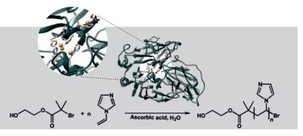
Enzymatic ATRP of N-vinylimidazole. The structure of the enzyme laccase shows the four copper atoms of the active site in orange and the amino acid residues that tightly complex the metal ions (graphic: N. Bruns)
