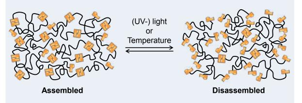
Schematic representation of the reversible disassembly of supramolecular polymers using light or heat (graphic: C. Heinzmann).
