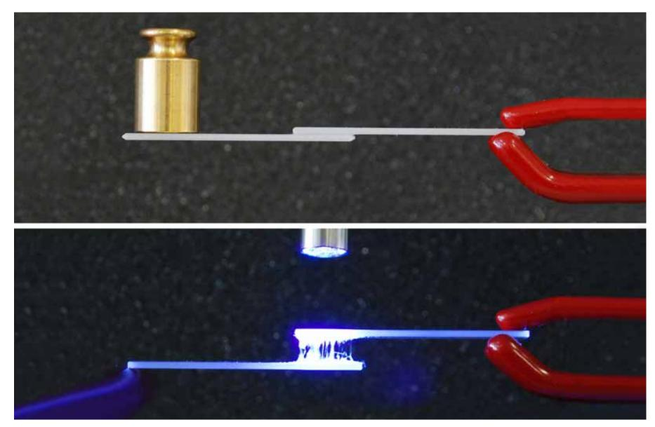
Visualizing the light-induced debonding feature of the supramolecular polymers used by AMI researchers. Under ambient conditions, the materials are powerful adhesives (top), whereas they liquefy and lose their adhesive properties upon heating or irradiation with ultraviolet light (bottom) (pictures: C. Heinzmann).
