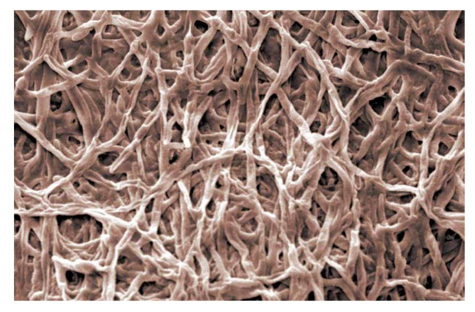
Scanning electron microscope picture of poly-butyl acrylate particles combined with β-lactoglobulin fibrils (picture: S. Rima)
