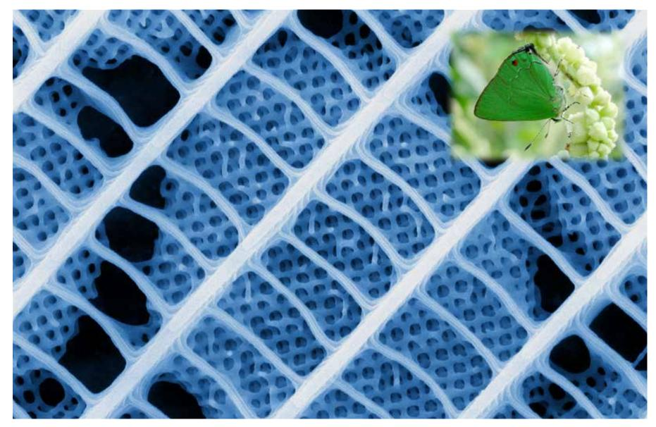
The ultrastructure of butterfly wing scale of the green-colored butterfly, *Erora opisena*, from Mexico (inset, picture copyright K. Garwood). Light interaction with these gyroid-structured networks in the scales result in the stunning green colour of these insects. (main picture: B. Wilts)
