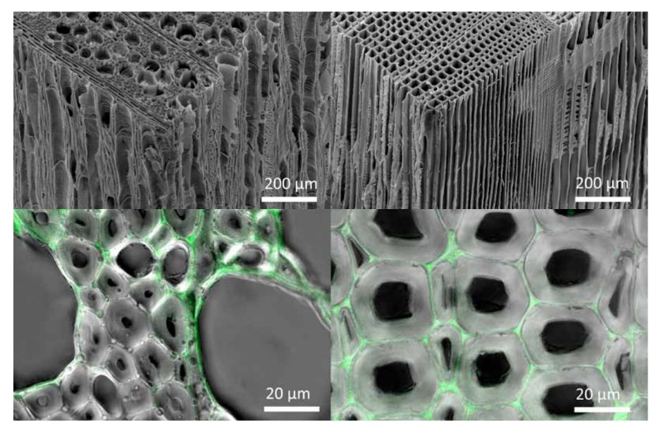
Top: scanning electron micrograph of beech (left) and spruce (right); Bottom: laser scanning image of beech (left) and pine (right) wood. The green overlay shows an auto fluorescence signal of lignin at an excitation wavelength of 488 nm (pictures: C. Geers)
